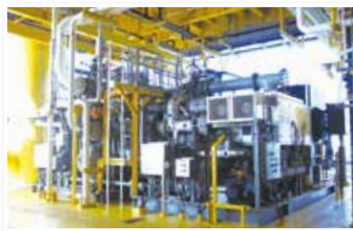
Vapor recovery compressor - Vietnam offshore 3225MMC / 600kW
